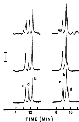
Figure 2. Traces from the HPLC experiments using \text{CH}_3\text{CN} (left) or \text{CH}_3\text{OH} (right) as solvent: (top) noncrystalline \text{B}'_{12} ; (middle) crystalline \text{B}'_{12} ; (bottom) mixture of d-, b-, and e-monocarboxylic acids. The vertical bar corresponds to 0.01 absorbance unit. HPLC separation conditions: 4.6 \times 250 mm Microsorb \text{C}_{18} ( 5 \mu\text{m} ) column; 15–20- \mu\text{L} injections of 0.34 mg/mL solutions (except for the crystalline \text{B}'_{12} , which was available in insufficient quantity for weighing); absorbance at 260 nm, 0.2 AUFS; flow rate 1.5 mL/min; 30-min gradients; solvent 0.1 M triethylamine/acetate buffer (pH 7.0); gradients from 10 to 15% \text{CH}_3\text{CN} (left) and from 20 to 25% \text{CH}_3\text{OH} (right). Separations were optimized by starting from conditions outlined by Jacobsen. 11
